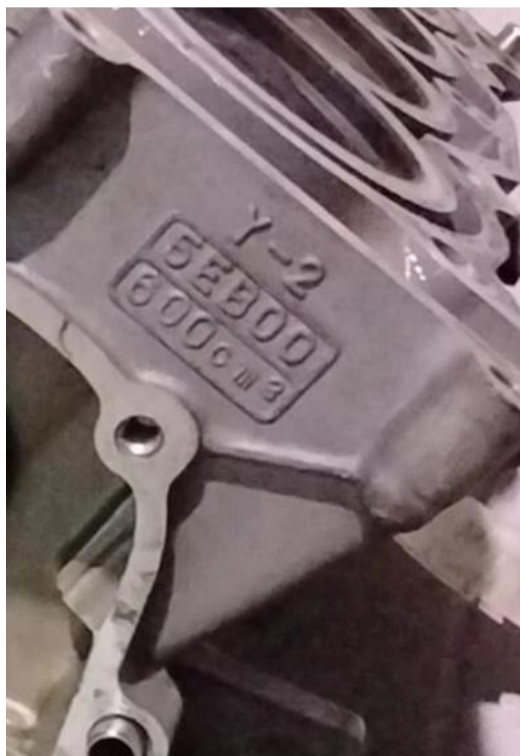
Incorrect 5SL crankcase (not to be used)
