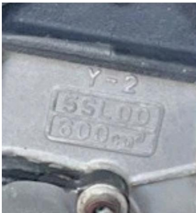
Incorrect 5SL crankcase (not to be used)
