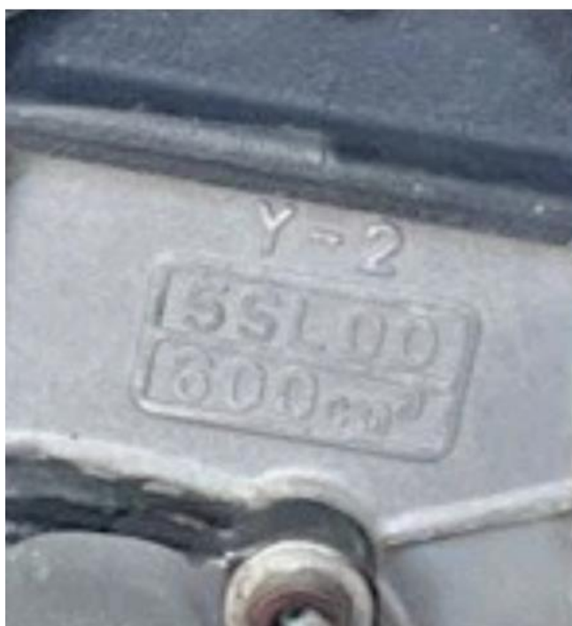
Incorrect 5SL crankcase (not to be used)
