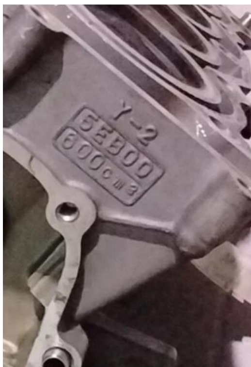
Incorrect 5SL crankcase (not to be used)
